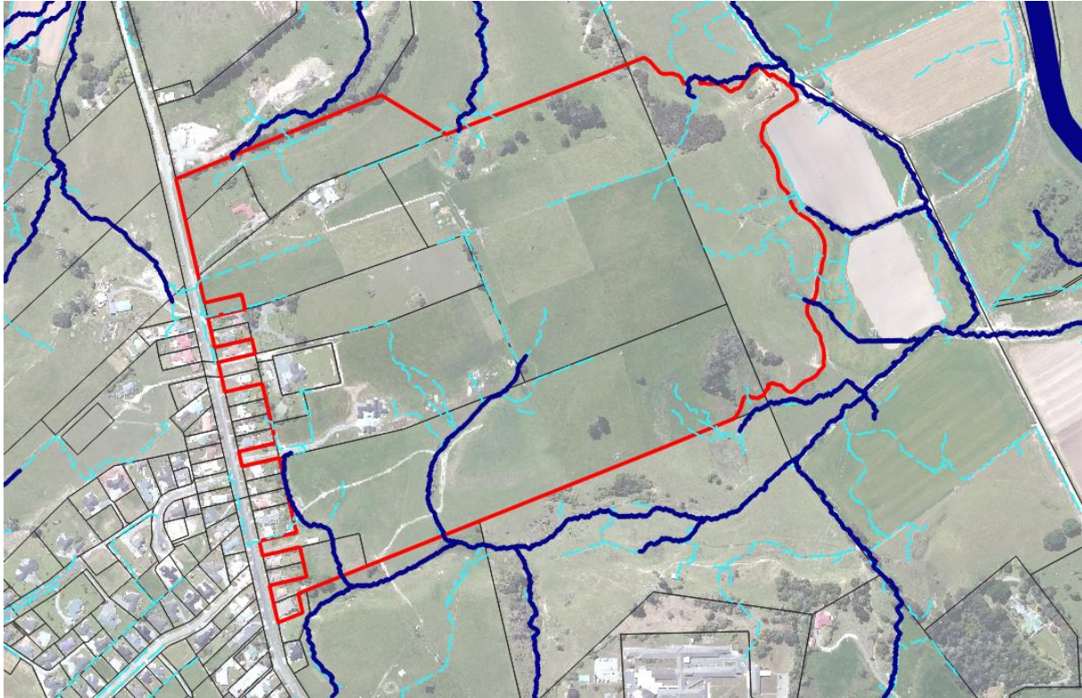
Figure 3-6: Sheetflow estimated in light blue dash lines and channelised flows in dark blue lines (please note flow path assessment above is indicative only as assessment uses LiDAR data which does not accurately capture culverts).
